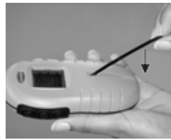
3. Place tip of strip in back end of channel, lay flat, pad side down. DO NOT SLIDE THE TEST STRIP ACROSS THE GLASS
