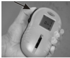
1. Press Power ON Turn Unit ON by pressing power button. Display will read "0"
